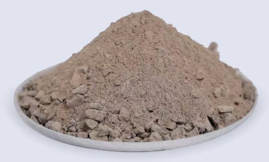
Ramming mix for EAF bottom is made of fused magnesia or medium-class magnesia and Mgo-CaO-Fe<sub>2</sub>O<sub>3</sub> sinter. It is characterized by high density, high strength, great resistance to corrosion, great thermal resistance, and long service life.
